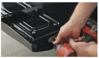
Step 15) Insert the tailgate brackets behind the tailgate latches and re-insert the bolts through both layers
