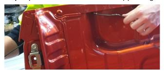
**Step 11)** Use the provided wire taps to connect the canopy wires onto the wires shown below. Red > Red Black > Black
