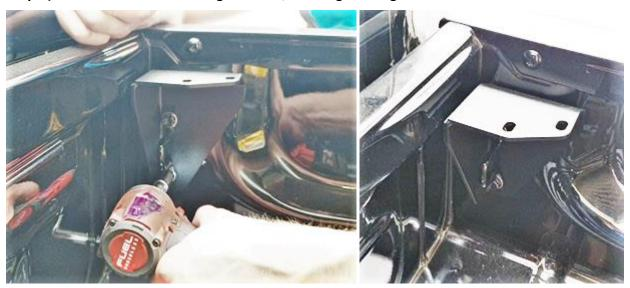
Step 4) Install the rear mounting brackets, re-using the original bolt
