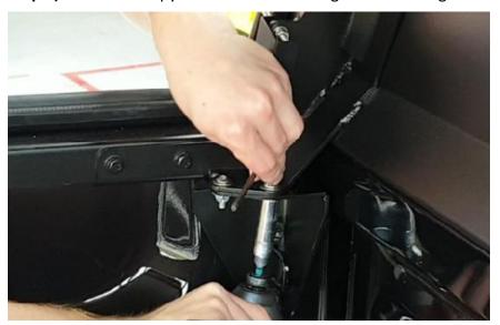
Step 7) Bolt the canopy to the rear brackets using the short M6 bolts, nuts, and washers
