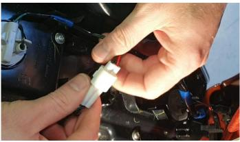
Step 10) Feed the wire from the canopy through the wellside into the rear light cavity
