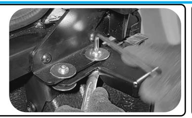
Bolt the canopy to the rear mounting brackets using the following fasteners:
