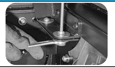
Bolt the canopy to the front mounting brackets using the following fasteners:
