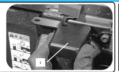
Install rear mounting brackets (1), these will cover the cut liner.
