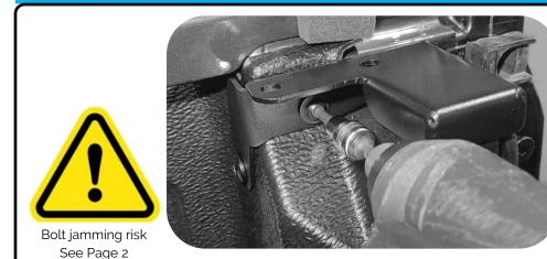
Re-install the original bolts through the brackets into the vehicle threads.
