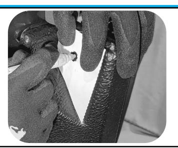
Sit the paper template on the liner in the rear corners, and mark the hole position.
