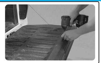
Remove the top row of screws from the tailgate.
