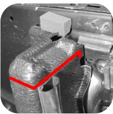
Mark around the liner at the top of the rear corners following the lines indicated.
