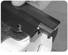
Sit the tailgate bracket PRT-005987 (12) in position, so the end tabs hook underneath the plastic liner.
