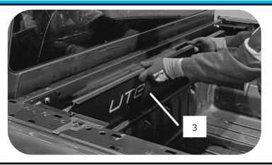
Lift the front panel (3) into position, ensure the base sits behind the plastic liner.
