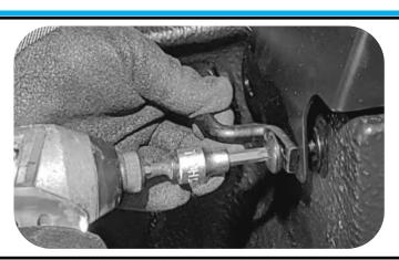
Re-install the front hooks through the corner plates.
