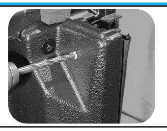
Drill through the mark with a 8.5mm drill bit.
