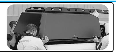
Lift the canopy onto the vehicle.
