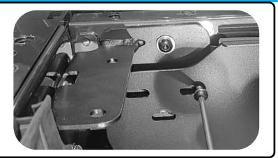
Bolt the front panel to the front mounting brackets using the following fasteners:
