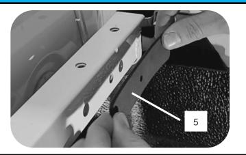
Install foam gasket (5) to the front wall over the threads.
