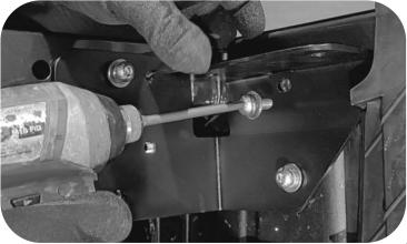
Install the front mounting brackets (2) using the following fasteners:
