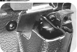
Cut around the marks from the previous step, to remove the top cap of the liner.
