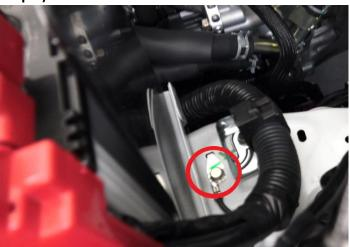
Step 3) Connect the earth cable to the earth point and re-install the bolt
