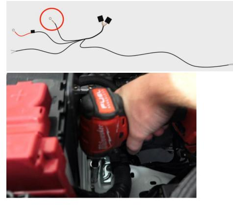
Step 4) Open the battery cover and remove the nut shown
