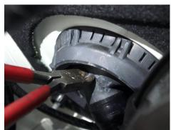
Step 9) Push the Lock/Unlock cable through the incision, locate on the interior and pull the slack through
