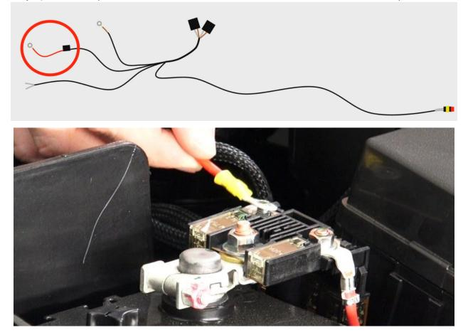
Step 6) Run the Lock/Unlock cable across to the driver's side. Leave cable loose at this stage
