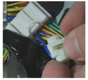
Step 13) Identify the wire labelled 'Lock\_Sig' and insert this into the plastic clip alongside the Blue/Black wire
