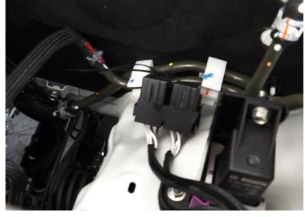
IMPORTANT: Ensure the relays are the correct way up (not upside down)
