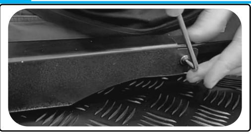
Bolt the front feet to the Side Rail thread plate, using the following fasteners:
