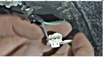
Step 4) Take the provided wiring loom and insert the black wire into the white clip
