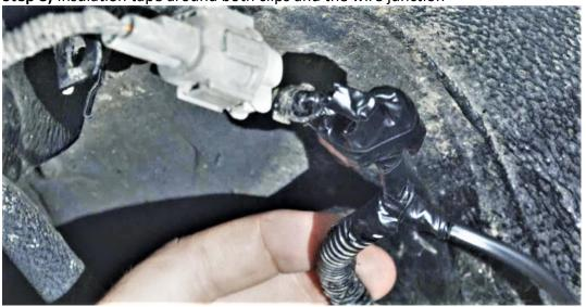
Step 9) Feed the plug end of the wiring loom over the fuel filler and up to the front corner of the wellside
