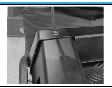
Bolt the front feet to the Load Stop using the following fasteners:
