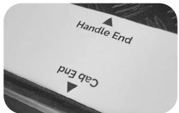
Ensure the template is oriented the correct way around. "Handle End" should be pointing towards the Load-Lid handle.
