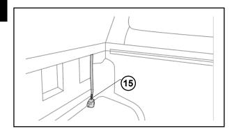
Remove the bolt and bump stop from the side of the tailgate.
