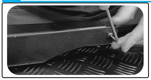
Bolt the front feet to the Side Rail thread plate, using the following fasteners:
