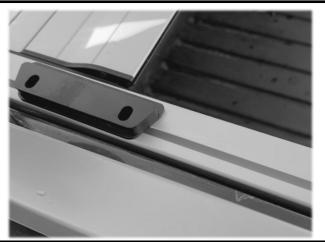
Place a large plastic packer [1] only on top of the **front** packer plates (the two closest to the sailplane)
