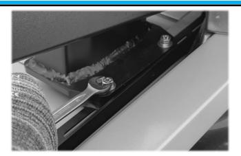
**Loosely** bolt down all the cantilever legs using the following fasteners:
