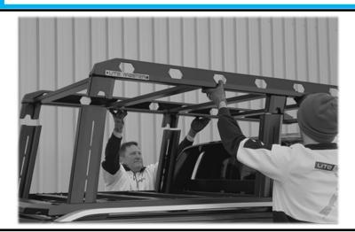
Sit the Cantilever Rack on top of the legs. You may need to reposition the legs to line up with the sockets on the rack.
