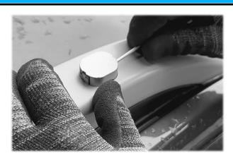
Remove the plastic cap on the roof rack using a small screwdriver.
