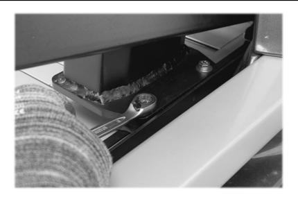
Tighten all the leg bolts now that the Cantilever is in its final position.
