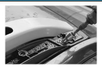
Remove the bolts holding the base plate down
