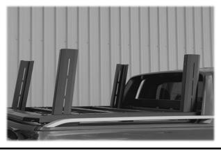
Place a Cantilever leg over each set of thread plates. 2x of the left leg will go on the left side. 2x of the right leg will go on the right side.
