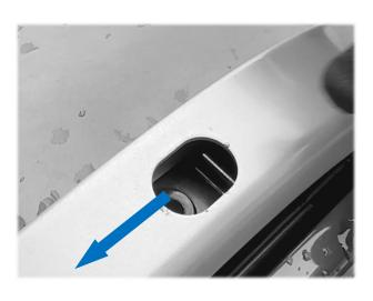
Slide the retainer plate backwards to release the roof rack
