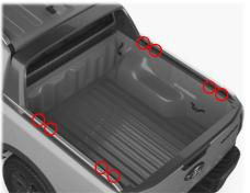
Slide 4x of the provided thread plates [8] in from the front of each track
