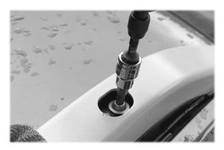
Remove the bolt using a T40 Torx bit.
