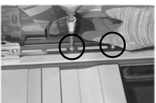
If you have a GearForce Tub Platform installed, remove the 4 indicated bolts on each of the base brackets.
