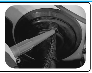
Seal the join where the wires enter the grommet tube.
