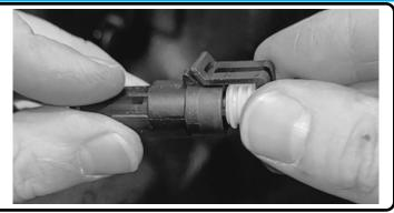
Connect the vehicle wiring loom to the Utemaster accessory inside the tray.
