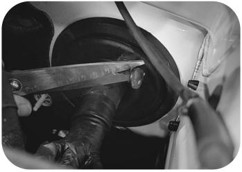
Identify the cab entry point on the passenger's side and cut the end off the tube.
