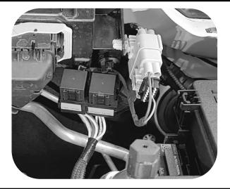
Cable tie the relays into the engine bay.
