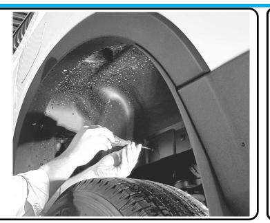
Remove all plastic clips from the rear passenger side wheel arch lining.
