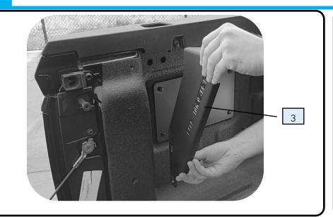
Install the rear mounting brackets PRT-006889 into the rear corners.
