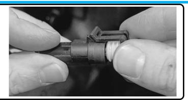
Connect the vehicle wiring loom to the Utemaster accessory inside the tray.
