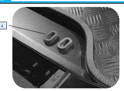
Place the foam gaskets PRT-004286 over the slots in the Load-Lid face plate.
