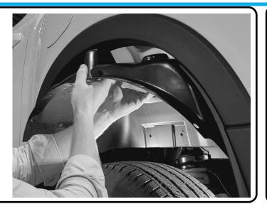
Re-install the plastic wheel arch liner, ensure all clips are returned to their original holes.
