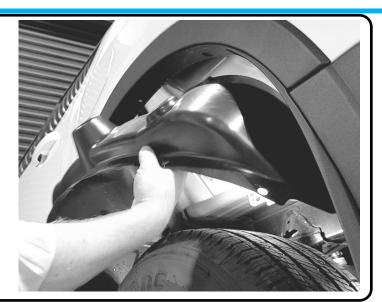
Remove the plastic wheel arch lining.
