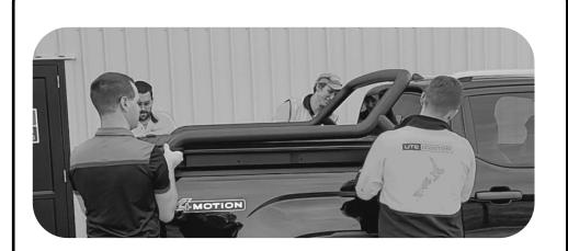
Lift the Load-Lid onto the vehicle.
