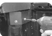
Install front sealing brackets on both sides using the following fasteners:
