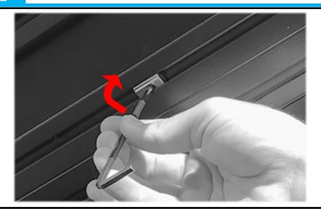
Rotate the T-nut over so the thread is facing out of the track. Using an Allen key or similar object is recommended for this step.
