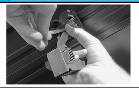
Using a 5mm Hex key, thread the cap screw into the T-nut thread plate. The holder should still be able to rotate
