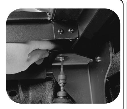
Bolt the Load-Lid to the front mounting brackets using the following fasteners:
