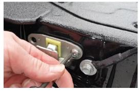
Step 7) Bolt the tailgate latches in using the original bolts, in the position shown
