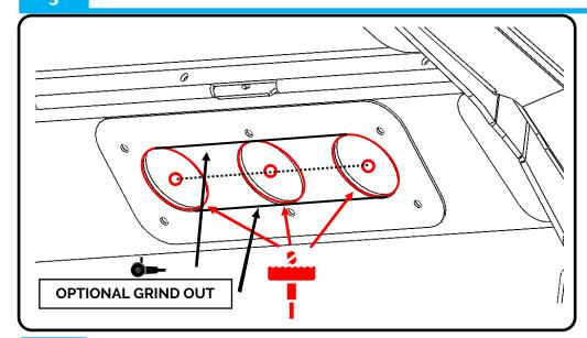
Using a 44mm Holesaw, drill out the 3x large holes using the pilot holes as a guide
