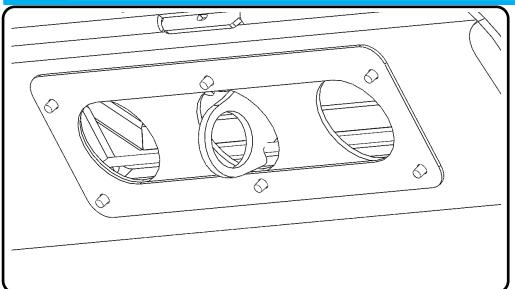
Place the cover plate [2] over the studs from the inside of the canopy
