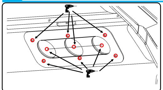
Drill out the 6x outside holes using a 5mm drill bit. Drill out the 3x inside pilot holes using the same drill bit
