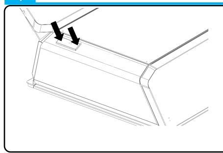
Place the Canopy Air Vent [1] over the hole cutout. Align the 6x studs on the vent with the 6x holes that were drilled out in step 3
