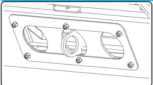
Bolt the Canopy Air Vent to the canopy wall using the provided 6x Nyloc nuts [4]
