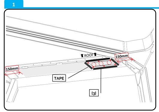
Tape the provided drilling guide [3] on the inside or outside front wall of your canopy as shown.
