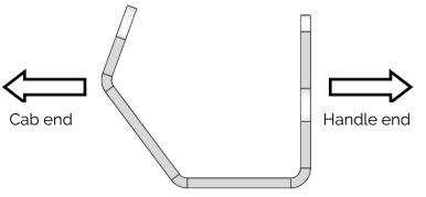
Ensure the base rail sits with the angled sides facing forwards towards the cab, and the flat side facing back towards the handle.
