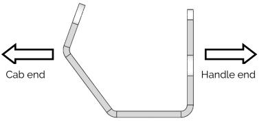
Ensure the base rail sits with the angled sides facing forwards towards the cab, and the flat side facing back towards the handle.
