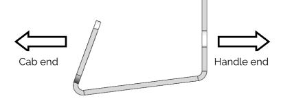
Ensure the base rail sits with the more angled side facing forwards towards the cab, and the flat side facing back towards the handle.
