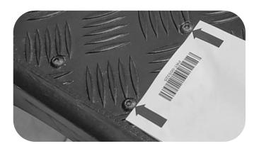
Ensure the arrows at each end are aligned with the hinge bolts. The template should sit centred on the Load-Lid, touching the bolts at each end.
