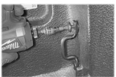
Remove the rear hooks on both sides of the tub
