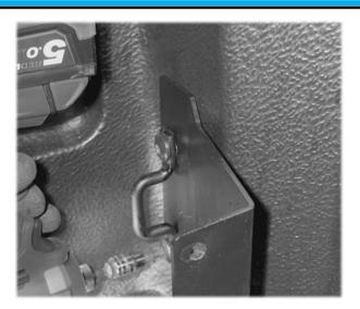
Reuse the bolts and install the rear brackets [2]
