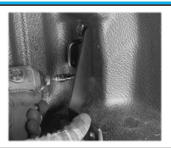
Reuse the bolts and install the front brackets [3]
