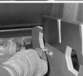
Loosely bolt the side boards to the brackets using the following fasteners:
