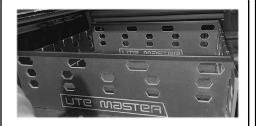
Place the central dividers at the front and rear positions to correctly space the sides
