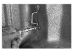
Remove the front hooks on both sides of the tub
