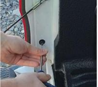
Step 17) Feed the wire from the canopy behind the mounting bracket and through the wellside into the rear light cavity
