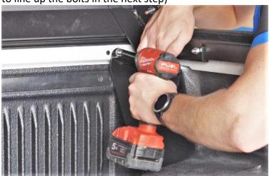
**Step 9)** Install M8 bolts into the two side wellside threads. Fully tighten all three bolts in the bracket
