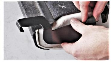
Step 16) Remove the rear light on the passenger's side of the vehicle
