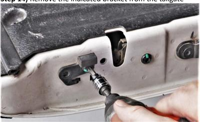
Step 15) Replace the tailgate bracket, sit the provided bracket on top, and bolt through both
