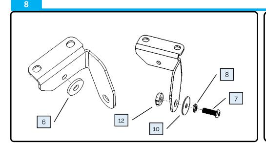
Pre-thread the following fasteners through the rear mounting bracket PRT-005979 (2).
