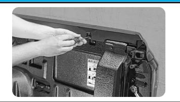
Remove the clips along the side of the plastic caps.
