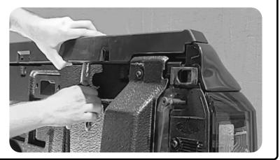
of the wellside. The clips need to have at least one side pushed inwards to release the clip.
