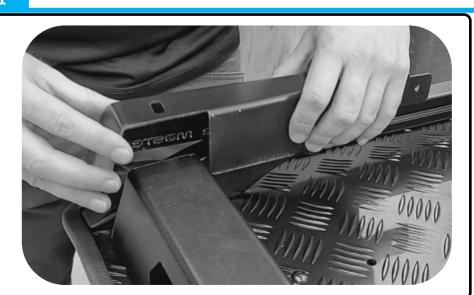
Sit the front feet (3) over the Load-Stop and Side Rail.
