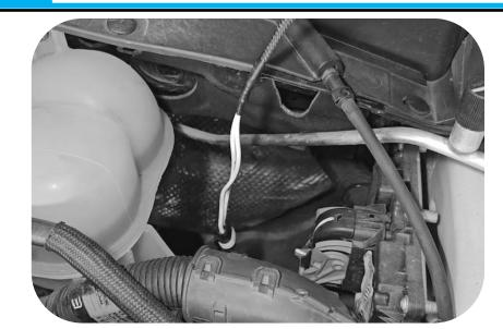
Feed the long cable down the firewall on the Passenger's side, to the underside of the vehicle.
