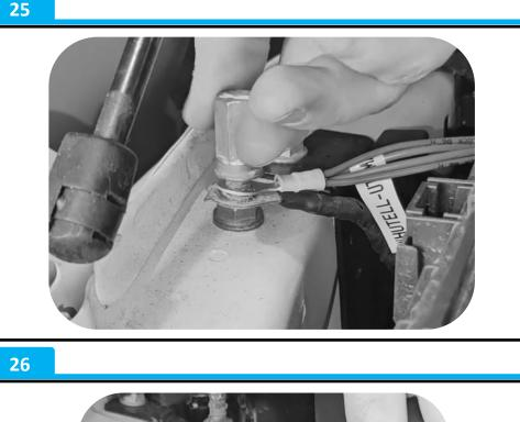
Connect the Ground cable to the ground connector on the vehicle
