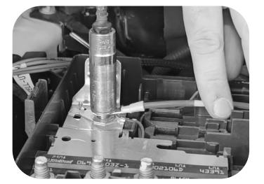
Connect the Power cable to the battery positive terminal
