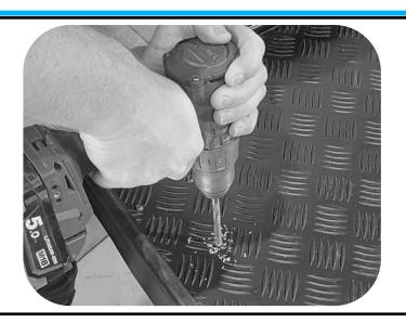
Drill through all marks with a 8.5mm drill bit.
