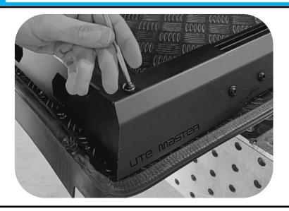
Bolt the front feet to the Load Stop using the following fasteners:
