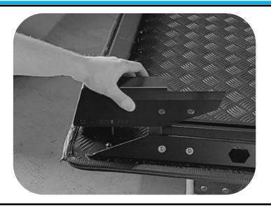
Sit the front feet (3) over the Load-Stop and Destroyer Side Rail.
