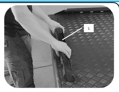
Sit the base rail (1) onto the front of the Load-Lid.
