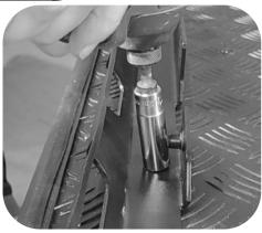
Bolt the base rail to the Load-Lid through each drilled hole using the following fasteners:
