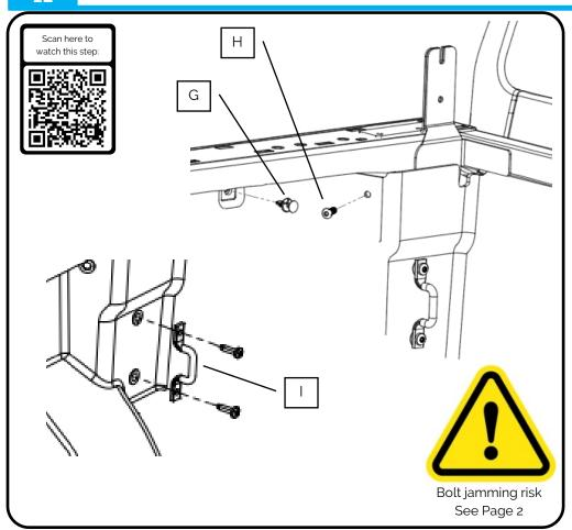
Remove the front clip (G) and bolt (H) holding the liner in the front corner.
