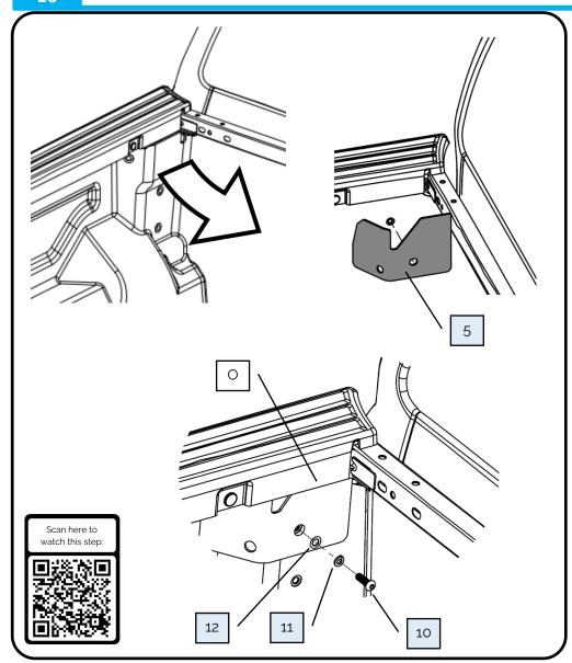
Pull the front corner of the liner away from the wellside wall to give access behind.
