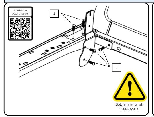
Remove the bolts (J) holding the sports bar bracket into the front corners.
