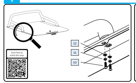
Bolt through the Load-Lid face plate into the rear feet using the following fasteners:
