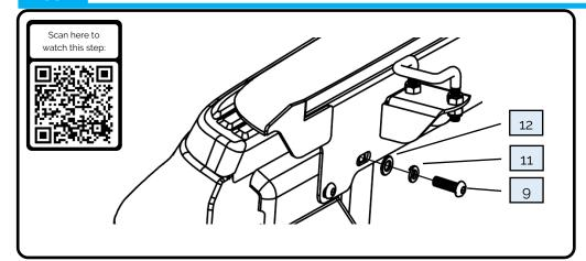
Bolt through the mounting frame into the rear mounting brackets using the following fasteners:
