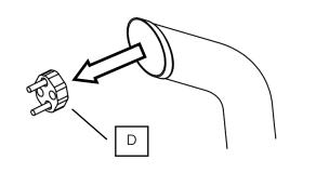
Remove the stud plates (D) from under the rear sports bar feet.
