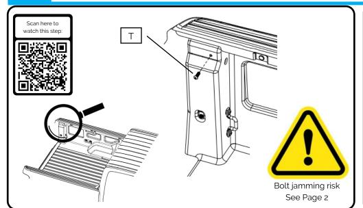
Remove the existing bolt in the top rear rear corner of the wellside (T).
