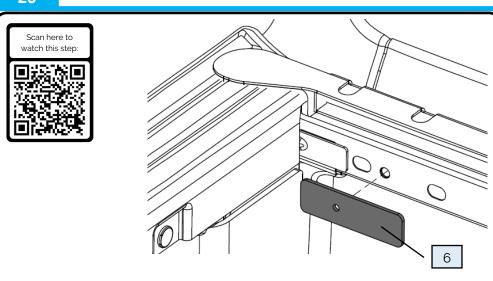
Install PRT-005963 onto the front wall to cover up the open slotted holes.
