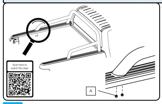
Remove the nuts holding the rear sports bar feet (A).
