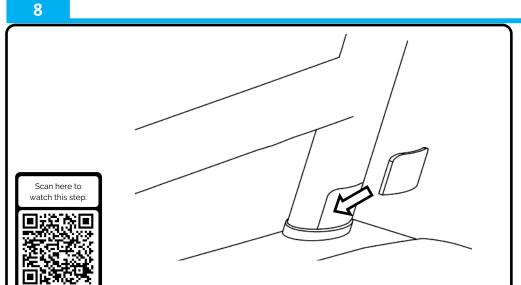
Re-install the rubber infill to the front sports bar feet.
