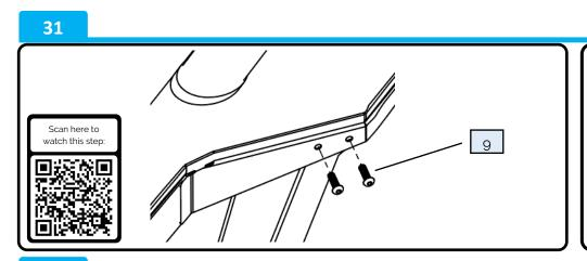
Bolt the centre bracket to the Load-Lid using the following fasteners:
