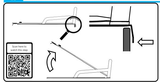
Ensure the Load-Lid is pulled backwards until the front flange touches the front face of the tray.
