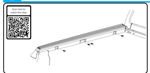
Remove the clips along the side of the plastic caps.
