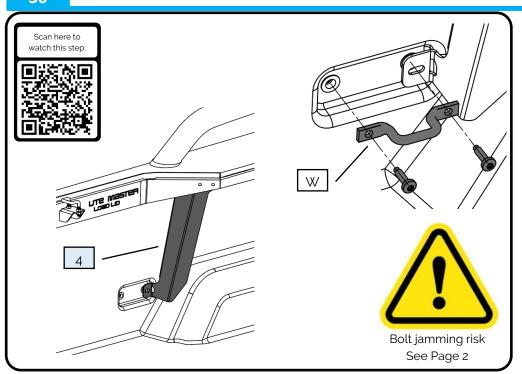
Install the centre mounting brackets PRT-005480-03 to the centre threads using the original hook and bolts (W).
