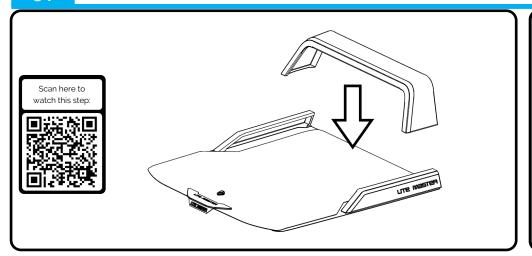
Lift the top hoop of the sailplane onto the Load-Lid.
