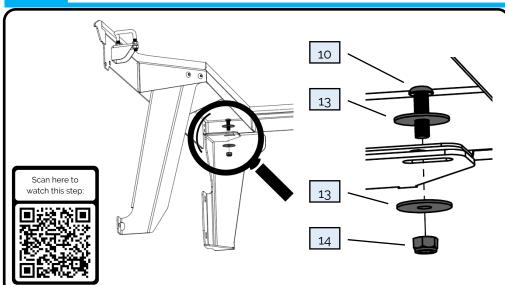
Bolt through the front corner of the Load-Lid into the front mounting bracket, using the following fasteners:
