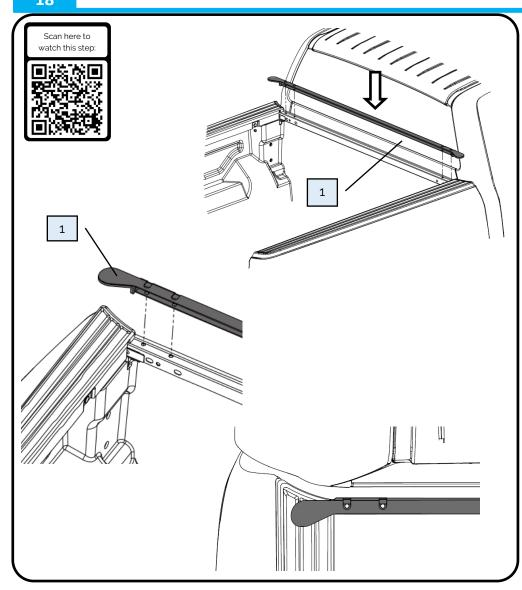
Install the front infill bracket PRT-005957-01 to the front wall of the wellside, between the two plastic caps.
