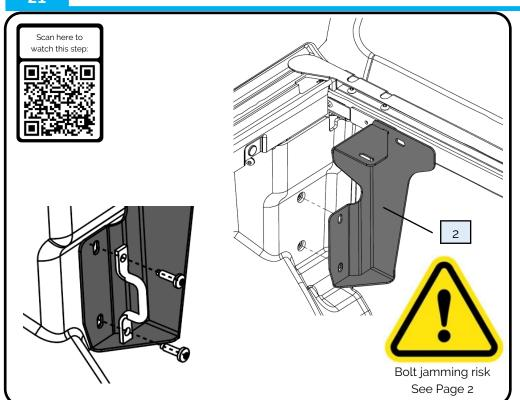
Install the front mounting brackets PRT-005962 into the front corners.
