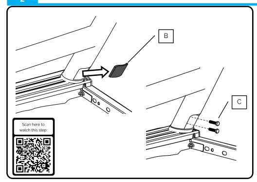
Remove the rubber infill (B) from the front sports bar feet.
