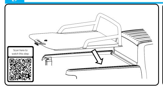
Lift Load-Lid onto the vehicle.
