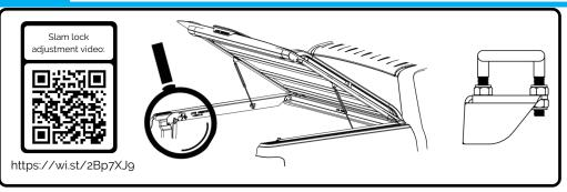
Adjust the nuts on the lock strike to affect the final closing height of the Load-Lid.
