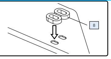
Place the foam washers (8) over the holes in the Load-Lid face plate.
