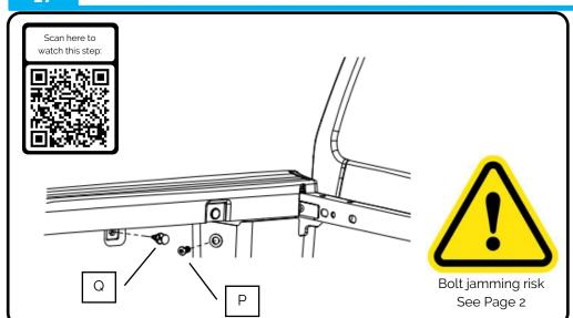
Return bolt (P) to it's original thread, ensure this passes through the hole in the rubber gasket.
