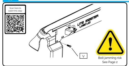
Insert the original bolt from Step 25 (V) through the mounting frame into the vehicle thread.
