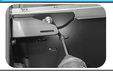
Bolt the front liner infill to the mounting brackets, using the following fasteners:
