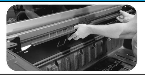
Install the front liner infill.
