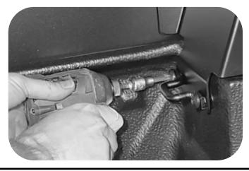
Re-install the hooks through the corner brackets.
