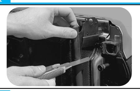
Trim down the bulb seal at the rear corner of the liner.
