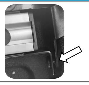
Re-install the T-Tracks using the original fasteners and brackets.
