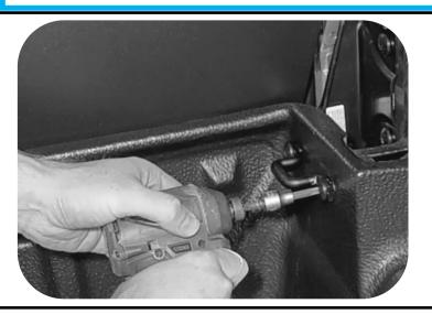
Once the Load-Lid is installed, remove the front hooks.
