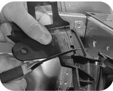
Peel back and trim the rubber brackets in the front corners.
