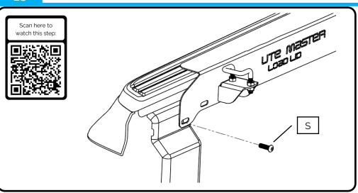
Without moving the Load-Lid, reach in through the open tailgate and insert the original bolt from Step 12 (S) through the mounting frame into the wellside thread.
