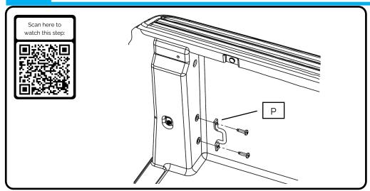
Remove the hooks from the rear corners (P).
