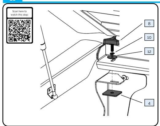
In the front corners, bolt through the mounting frame and front mounting bracket into the provided thread plate, using the following fasteners:
