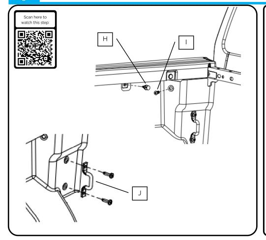
Remove the front clip (H) and bolt (I) holding the liner in the front corner.
