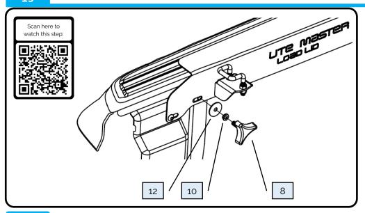
Reach through the open tailgate and bolt through the mounting frame into the rear mounting bracket using the following fasteners:
