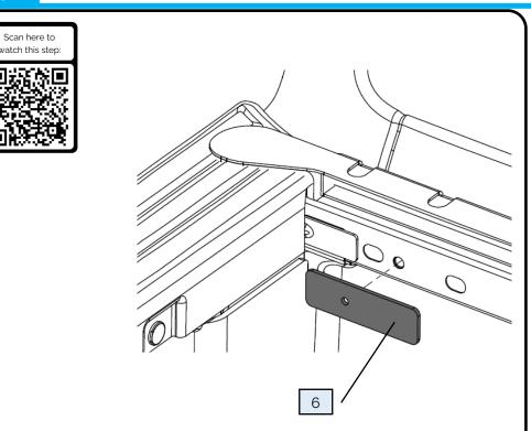
Install PRT-005963 onto the front wall to cover up the open slotted holes.
