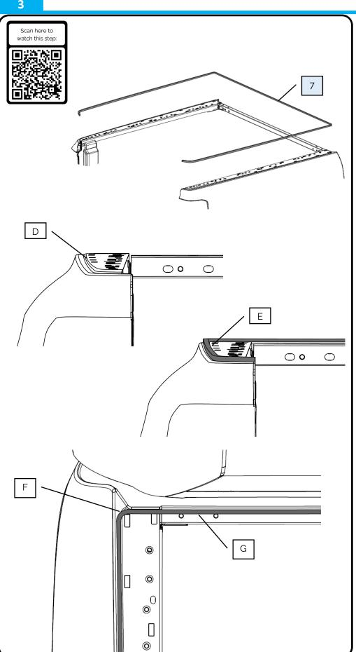
Run the provided sponge seal around the outside of the wellside in a continuous seal, starting at the tailgate on one side and ending at the tailgate on the other side.
