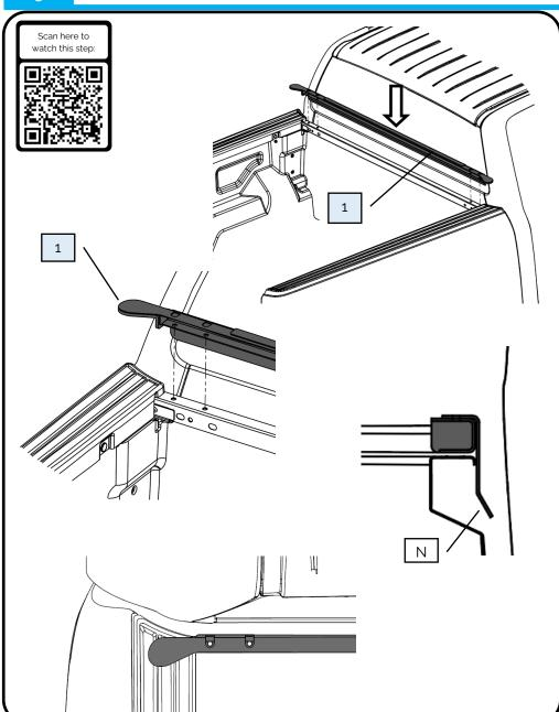
Install the front infill bracket PRT-005957 to the front wall of the wellside, between the two plastic caps.
