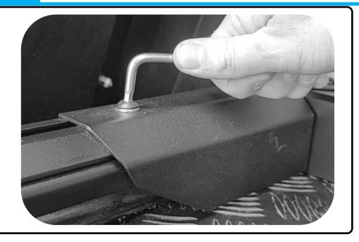
Bolt the front feet to the Side Rail thread plates using the following fasteners:
