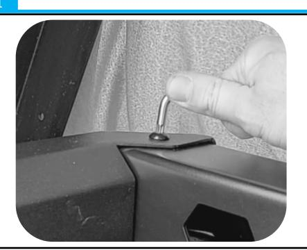
Bolt the front feet to the Load Stop using the following fasteners:
