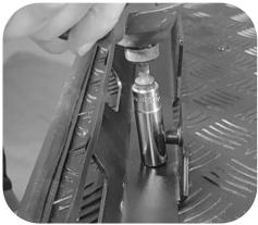
Bolt the base rail to the Load-Lid through each drilled hole using the following fasteners:
