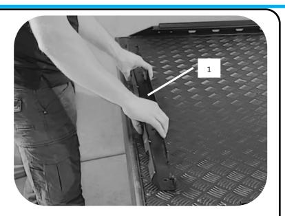
Sit the base rail (1) onto the front of the Load-Lid.
