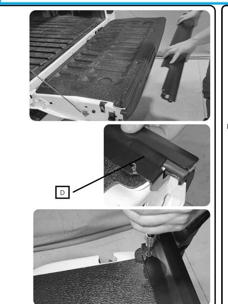
Sit the tailgate bracket PRT-005987 (1) in position, so the end tabs hook underneath the plastic liner.
