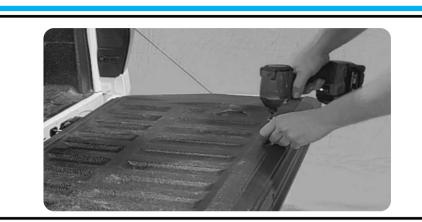
Remove the top row of screws from the tailgate.
