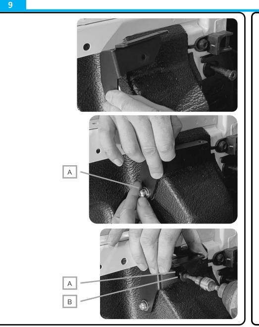
Install the rear mounting bracket PRT-005979 (2) using the fasteners listed in the previous step.
