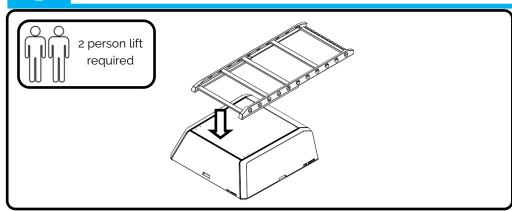
Fit cantilever onto the canopy roof.
