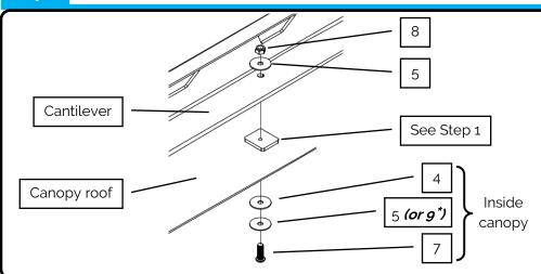
Bolt both front corners using the following fasteners:
