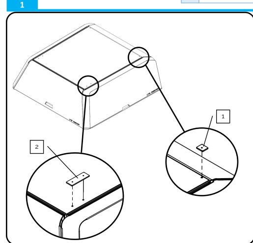
NOTE: the canopy may have blanking bolts in these holes. Remove these bolts before proceeding with the installation.
