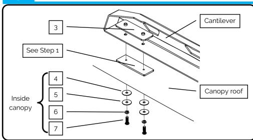
Bolt both rear corners using the following fasteners:
