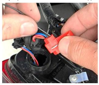
Step 22) Squeeze the clip until the metal paddle is flush with the plastic.
