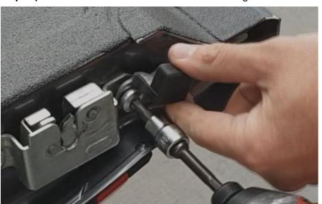
Step 15) Assemble the bracket with the provided tailgate brackets, with a washer in between so the tailgate bracket sits flat. Use a bolt to hold them together before installing to the tailgate.
