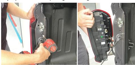
**Step 18)** Feed the brake light wire from the canopy through into the tail light cavity.
