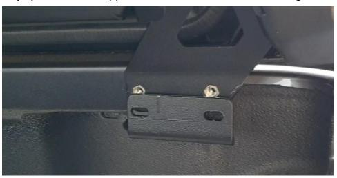
Step 9) Bolt through the rear mounting bracket into the threads in the canopy.
