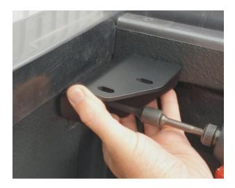
**Step 4)** Remove the bolts from the rear corner of the wellside.
