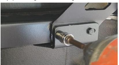
**Step 10)** Bolt the canopy to the front mounting brackets.
