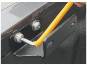
Step 6) Remove the bolts in the rear corners of the canopy.
