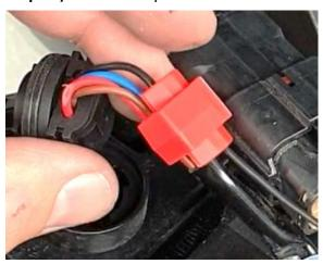
Step 24) Repeat Steps 20-23 to attach the red canopy wire to the red tail light wire.
