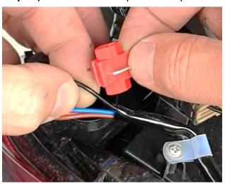
Step 21) Feed the black wire from the canopy into the clip alongside the black light wire.
