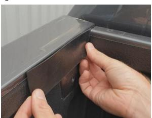
Step 3) Install the front mounting brackets. Passenger side is marked with 'PS' and driver's side is marked with 'DS'.
