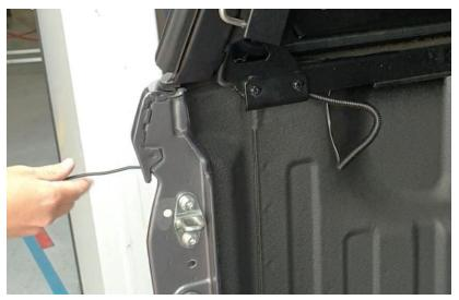
**Step 19)** Splice the end of the wire to reveal the individual red and black wires.
