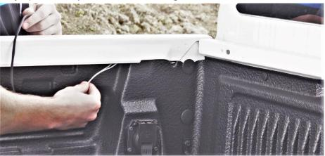
Step 3) Pull the wire out below the fuel cap
