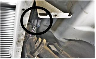
Step 5) Insert one of the white clips provided onto the purple wire
