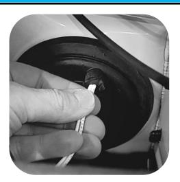
Feed the lock signal wires through the tube and pull out into the cab interior.
