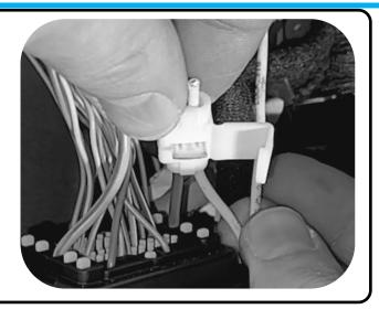
Insert the wire labelled 'Unlock\_Sig' into the white clip.
