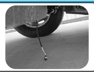
Feed the longest branch of the loom down the firewall to the underside of the vehicle.
