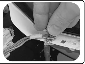
Install the ground terminal to the ground point above the firewall on the passenger's side.
