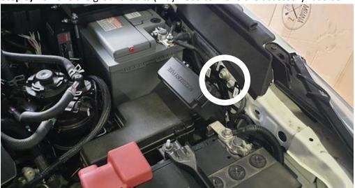
Step 4) Connect the ground cable to the ground point and re-install the bolt
