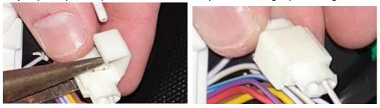
Step 16) Repeat Steps 13-15 to connect the wire labelled 'Lock\_Sig' to the Black wire
