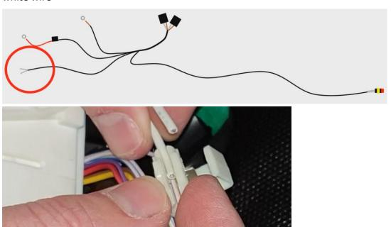
Step 15) Clamp the clip closed until the metal plate is no longer protruding, and close the clip
