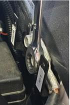
**Step 5)** Open the battery cover and remove the nut shown
