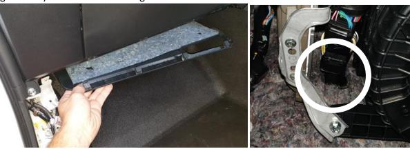
Step 10) Remove the plastic caps and rubber seal to expose the wiring behind the kick panel
