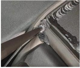
Step 33) Fill the hole in the front corner with sealer, ensure the sealer is pushed inside (not just sitting on the outside).
