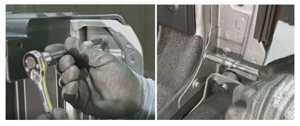
**Step 18)** Seal the join shown, between the drainage channel and the vehicle.
