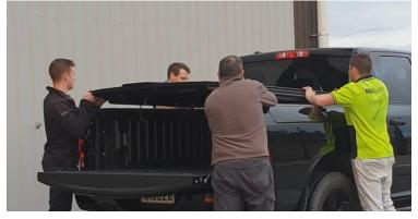
Step 29) Push the Load-Lid as far forward as possible. Test the tailgate to ensure it closes before proceeding to the next step.
