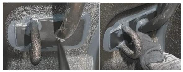
Step 17) Drop the tailgate and remove the two bolts shown below.
