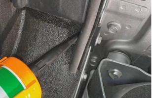
Step 27) Apply sealer to the junction where the three components meet (drainage channel, tailgate bracket, and vehicle).
