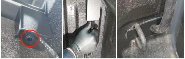
Step 15) Seal right around the hooks so there is no gaps for water to leak through, then seal around the edges of the plate. Wipe any excess sealer away so it looks tidy. (*Tip: use soapy* water to smooth the sealer and give a nice finish).
