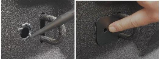
Step 35) Insert a black M8 bolt through the hole in the plate. Reach up underneath the vehicle and place an M8 fender washer and M8 nyloc nut on the bolt. Tighten up until it holds the plate firmly (two people required for this step).
