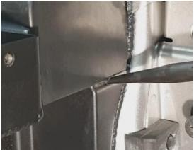
Step 21) Seal around the top along the join shown below.
