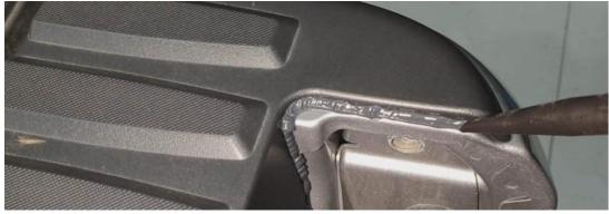
Step 22) Run sealer along the base of the plastic as shown.
