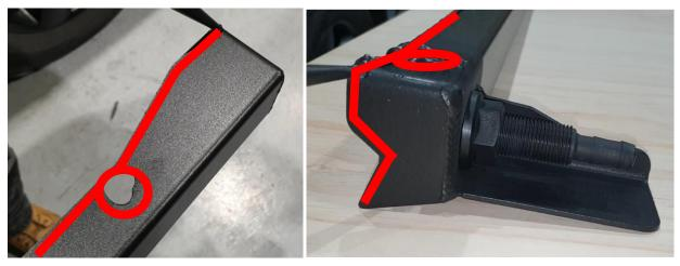
Step 7) Install the drainage channel to the vehicle, ensure it is pushed hard against the front wall with a good glue seal, and have the whole channel sitting as low as possible.
