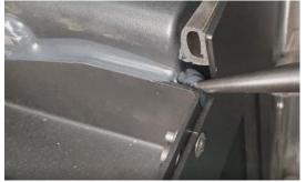
Step 28) Lift the lid onto the vehicle. Ensure the frame sits down inside the drainage channels.
