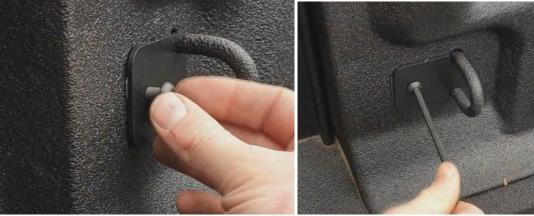
Step 36) Seal right around the hooks so there is no gaps for water to leak through, then seal around the edges of the plate. Wipe any excess sealer away so it looks tidy. (*Tip: use soapy* water to smooth the sealer and give a nice finish).
