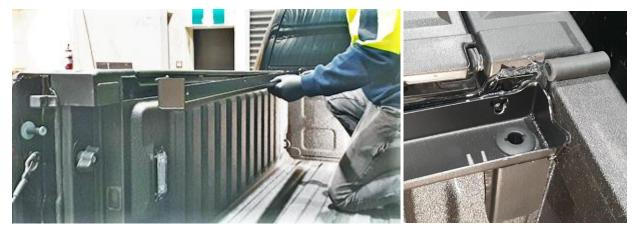
Step 8) Install two bolts through the drainage channel into the wellside threads, the thread in the front corner and the second thread from the rear. Use the original bolts which were taken from the sides in Step 2.
