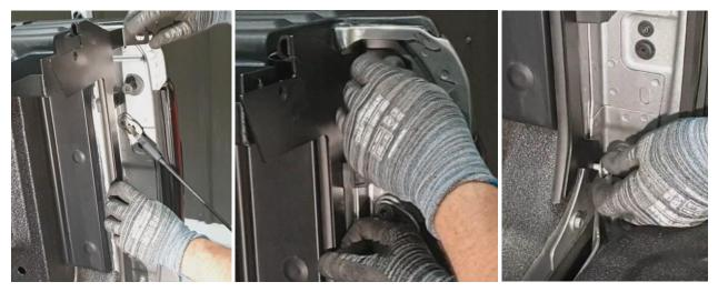
**Step 25)** Bolt the tailgate bracket to the drainage channel, then tighten the other two bolts.
