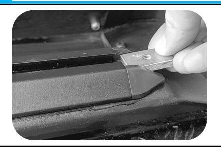
Insert the thread plates (7) into the Side Rail T-Tracks at the front of the Load-Lid.
