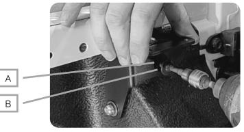
Install the rear mounting bracket PRT-005986 (2) using the fasteners listed in the previous step.
