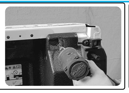
Remove the bolt in the rear corners.
