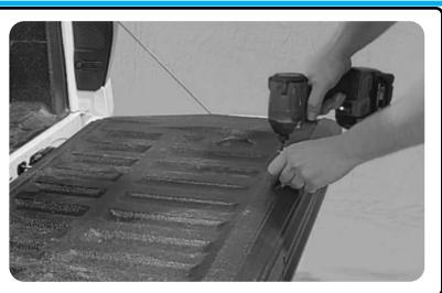
Remove the top row of screws from the tailgate.
