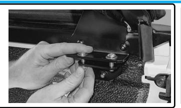
Bolt through the canopy into the rear mounting brackets using the following fasteners:
