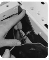
Pull back the liner in the front corners and install the rubber gasket PRT-005961 (4) behind.
