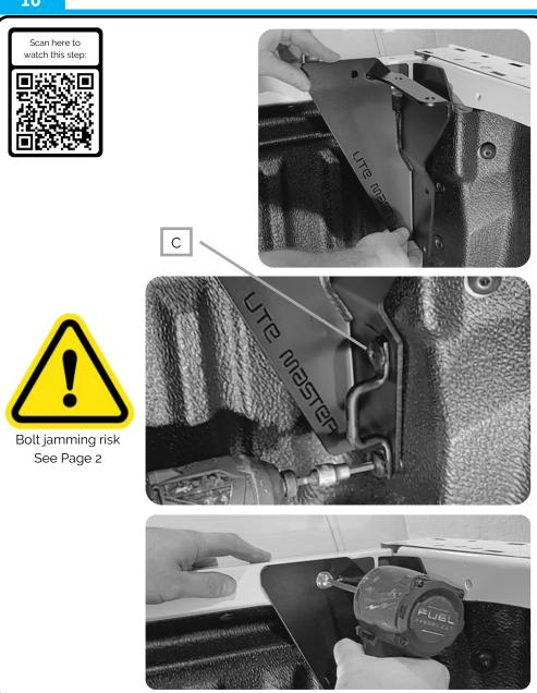
Install the front mounting bracket PRT-005600 (3) using the original hook and bolts (C).
