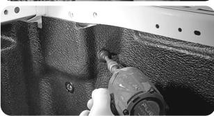
Re-install the front bolt through the liner, ensure it also goes through the second hole in the rubber gasket.
