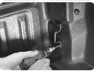
Remove the front clip and bolt holding the liner in the front corner.
