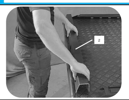
Lift the top rail (2) onto the base rail.
