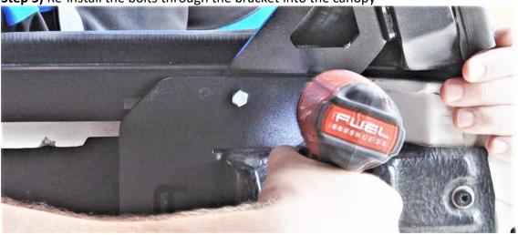
Step 6) Re-install the hooks with bolts going through the brackets
