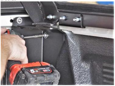
Step 10) Insert bolts connecting the canopy to the front bracket and fully tighten
