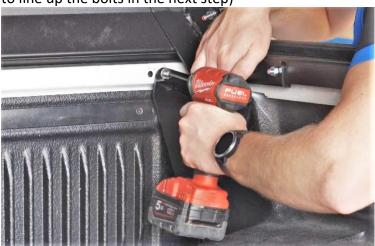
Step 9) Install M8 bolts into the two side wellside threads. Fully tighten all three bolts in the bracket
