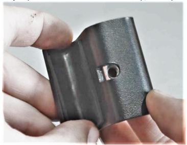
Step 13) Bolt through the top face into the barrel nut, pulling the clamp tight
