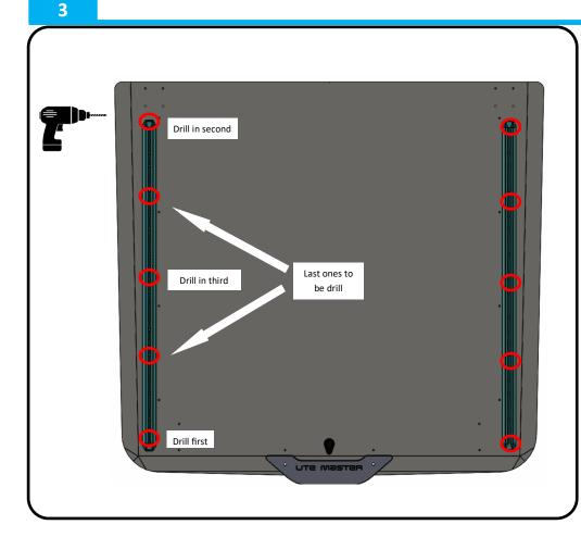
Drill 6.5 mm holes by beginning on the extremities ones. Then add a hole in the center of both extremities and one hole between center and each extremities.
