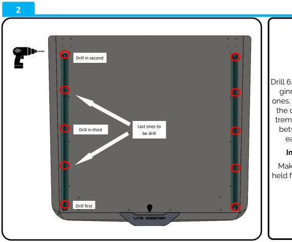
Drill 6.5 mm holes by beginning on the sides ones. Then add a hole in the center of both extremities and one hole between center and each extremities
