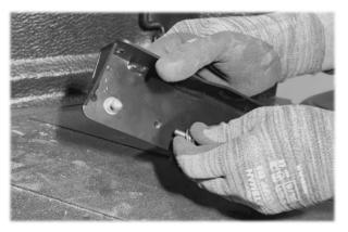
Loosely pre-assemble the rear bracket [1] to the clinch plate [2] using the following fasteners:
