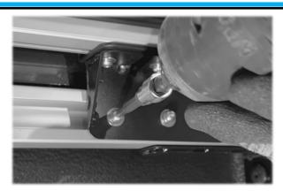
Tighten the clinch plate bolts to fully fix the bracket in place
