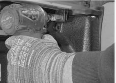
Remove the bolts fixing the small rear brackets in place
