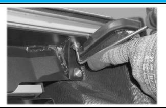
Tighten the loose top bolt using a 4mm Allen key
