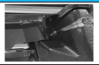
Slide the bracket all the way to the end of the rail and bolt in to the side hole using the following fasteners:
