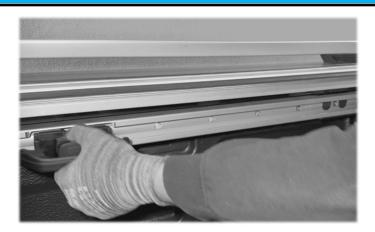
Remove the rearmost spring-loaded tie hook on both sides
