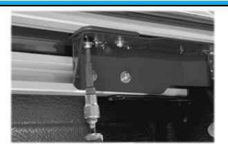
Bolt the rear bracket up into the top rail using the following fasteners:
