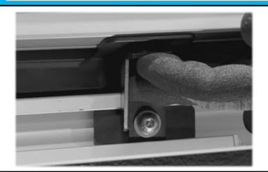
Slide the bracket into the front section of the rail
