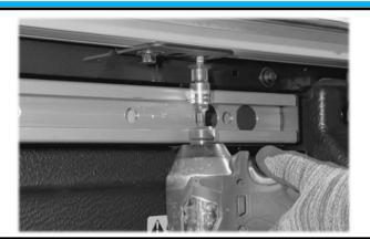
Remove the 2 factory bolts holding the rail angle bracket in place
