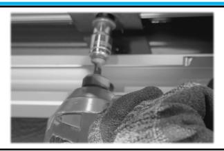
Remove the bolt from the front factory angle bracket
