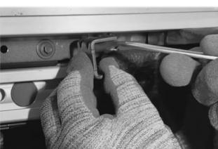
Remove the last bolt holding the remaining bracket in place.
