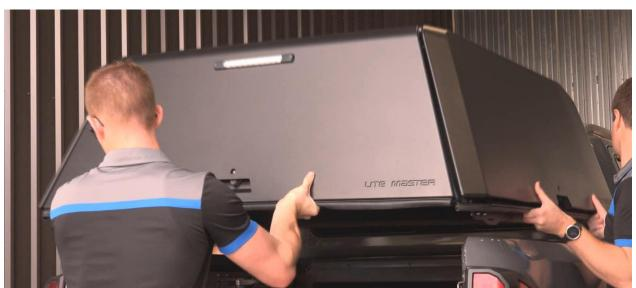
Step 11) Bolt the canopy to the front brackets, using M8 nuts and bolts with steel washers on both sides.
