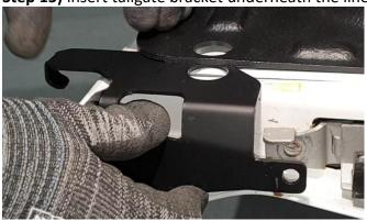
**Step 16)** Re-install the bolts through the tailgate bracket.
