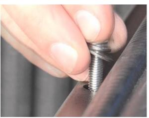
**Step 14)** Remove the tailgate latch bolt, and the liner bolt from the top corner of the tailgate (only if ute has a liner).
