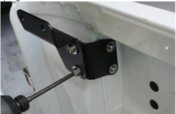
Step 8) Install the front brackets (PRT-004209) to the front wellside threads, ensure steel washers and spring washers are used with the bolts.
