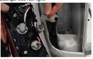
**Step 18)** Feed the canopy brake light wire through the wellside into the rear light cavity.
