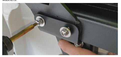
Step 13) Install the clamping tab (PRT-004440) to each side, with nyloc nut underneath the clamping tab.
