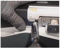
Step 17) Remove and unplug the passenger side rear light.
