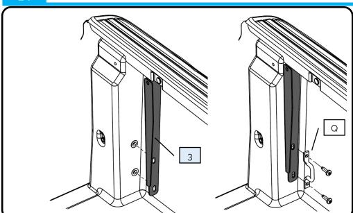
Install the rear mounting brackets PRT-005465 into the rear corners.
