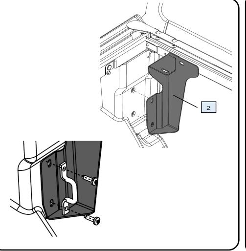
Install the front mounting brackets PRT-005962 into the front corners.
