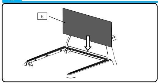
Insert cardboard (R) between the cab and wellside to protect the paint from scratching during installation.
