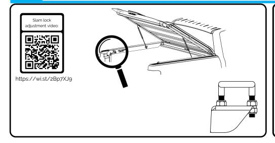
Adjust the nuts on the lock strike to affect the final closing height of the Load-Lid.
