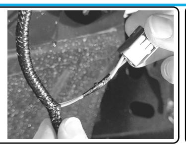
Peel back a section of conduit to reveal the two wires inside.
