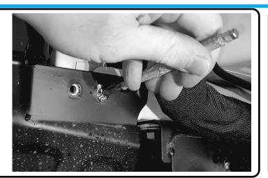
Clear any remaining rivet shafts from the holes.
