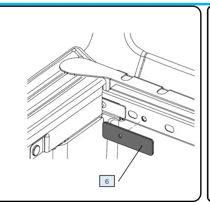
Install PRT-005963 onto the front wall to cover up the open slotted holes.
