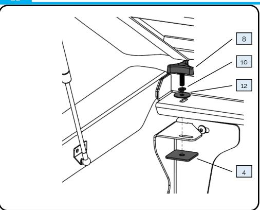
In the front corners, bolt through the mounting frame and front mounting bracket into the provided thread plate, using the following fasteners:
