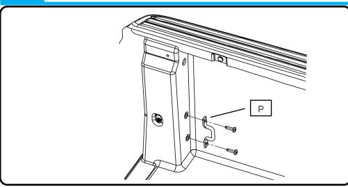
Remove the hooks from the rear corners (P).
