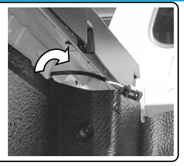
Locate the access point into the tray above the fuel cap, and feed the loose end of the wiring loom up into the tray area.
