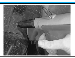
Rivet the plastic wheel arch liner in position through the original rivet holes, using the provided rivets.
