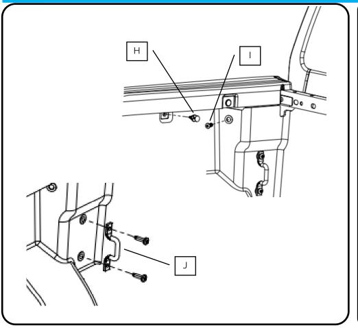
If you have a plastic wellside liner, remove the front clip (H) and bolt (I) holding the liner in the front corner.
