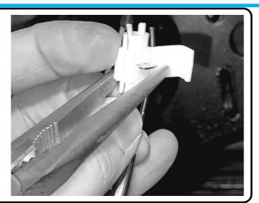
Squeeze the white clip with pliers until the metal clip sits flush with the plastic.
