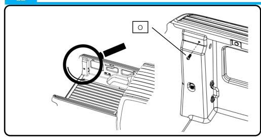
Remove the existing bolt in the top rear rear corner of the wellside (O).
