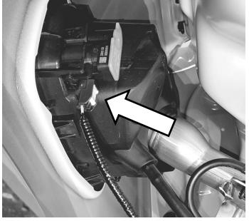
Locate and remove the fuel filler cap central locking plug.
