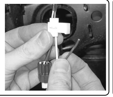
Feed the white wire from the end of the provided wiring loom 80606-26 into the white clip, alongside the white wire.
