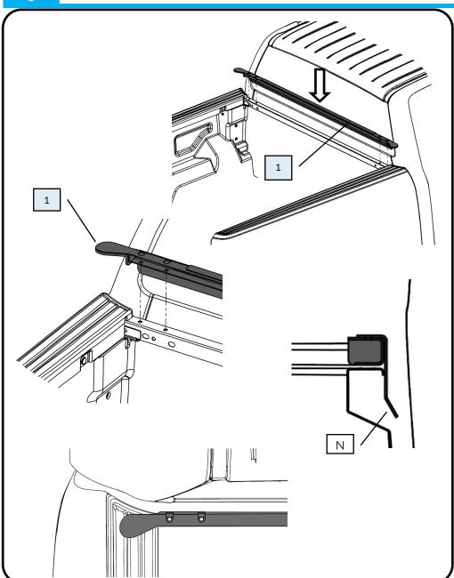
Install the front infill bracket PRT-006891 to the front wall of the wellside, between the two plastic caps.
