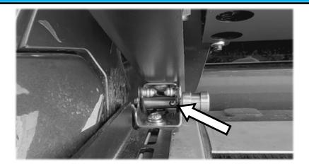
Insert the R-clip [12] into the pin hole to secure the platform
