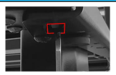
Adjust the rear lock catch to line up roughly in the middle of the adjacent slot in the platform. Once in position, tighten the two countersunk bolts that were left loose in step 6.
