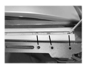
Slide the rear most thread plate all the way until it makes contact with the end. This thread plate dictates the final position of the bracket so ensure it stays hard against the rear.
