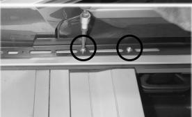
Bolt the base bracket [1] down to the thread plates in the 5 circled locations. Use the following fasteners:
