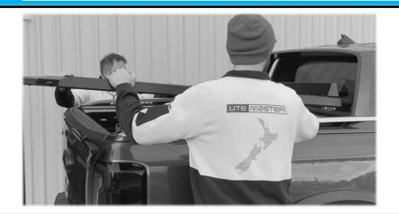
Place the assembled platform onto the base brackets. Make sure the Hinge brackets up the front have slotted in to each other.
