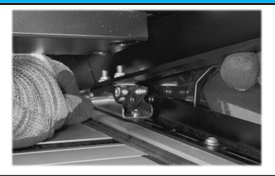
Slide in the hinge pins **[5]** on both sides.
