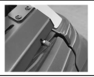
Open and close the platform to test whether the lock catches are in the correct position.
