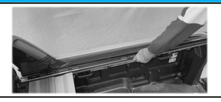
Line up the Platform base bracket [1] with the side of the track. This bracket will be used to get an approximate position for the thread plates in the next step
